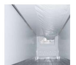
For added durability, Utility has changed the standard sidewall lining on all Utility refrigerated trailers to a "high impact" bi-directional fiberglass reinforced, polypropylene plastic lining. Over half of Utility customers are already utilizing this lining on the interior sidewall of their reefers because of its resilience and longevity compared to traditional F.R.P. linings.
